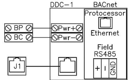
**Figure 37 - BACNET Connections**
