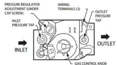
**Figure 23 – Modulating Valve**
