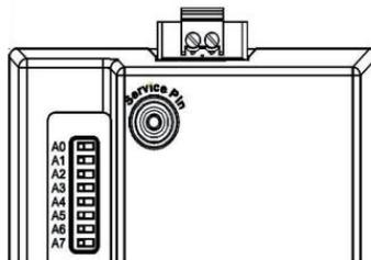
**NOTE: Insert Small Screwdriver. Tilt Toward LonWorks Port To Activate Service Pin.**
