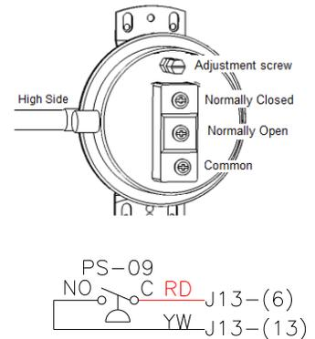
Figure 43 - Clogged Filter Switch and Wiring Reference
