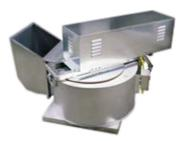
This fan is ideal for high temperature, solid fuel, and heavier grease applications. Select this fan over the TUSBI-RM model for applications that require a 500 °F temperature rating. Note that this temperature rating is only available for belt driven configurations; direct driven models are rated to 300 °F. The ability to tilt out this model's wheel for cleaning makes maintenance quick and easy. An upblast configuration is available which allows convenient ducting through the bottom of
