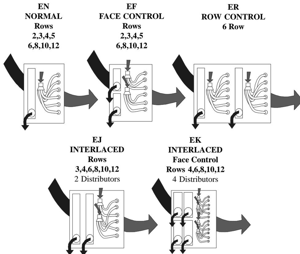
**Figure 1 - Evaporator Coils**
